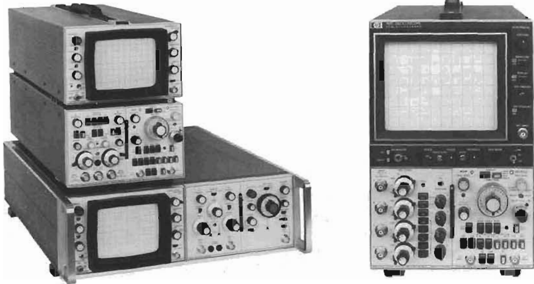
Figure 1. Representative plug-in oscilloscopes from Hewlett-Packard's 180 series.
