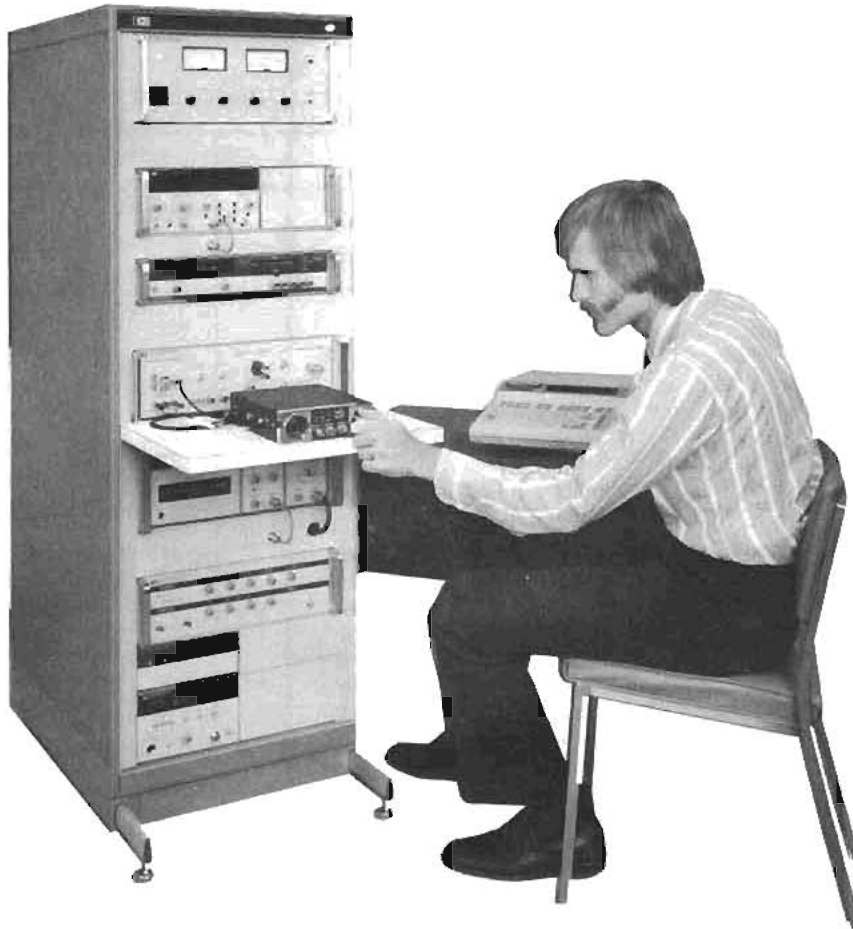
A preassembled HP-IB system solution — the 8950A Automatic Transceiver Test System.
