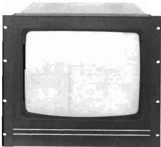
1317A with standard rack mount ears fits in 48.3 cm (19 in.) rack.
