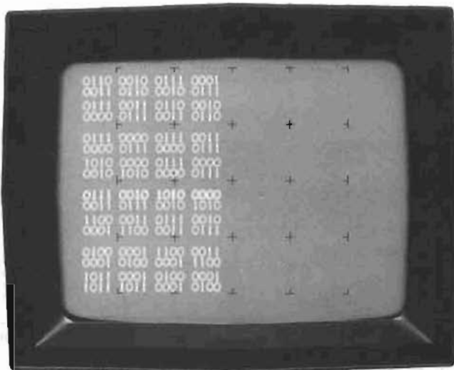
The digital memory may be used to capture events leading up to and including the trigger word (displays negative time). By also using delay mode, the end display trigger word may be positioned mid screen to display both negative and positive time data.
